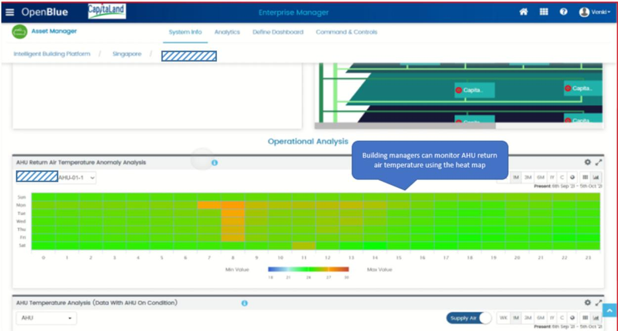
Figure 29. AHU Return Air Temperature Anomaly Analysis
