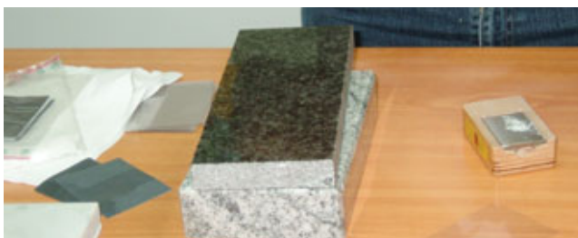
Fig. 9.6 – Sequences in natural stone rectification using wax fillers.
