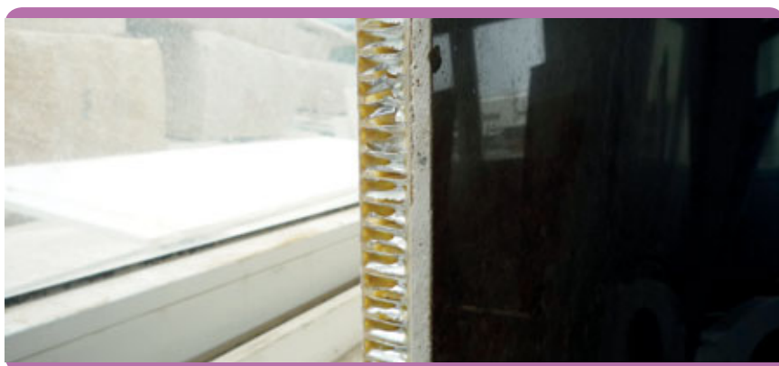
Fig. 4.1 – A cross-section of a typical aluminum honeycombed composite panel.
