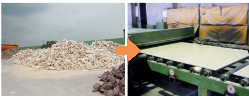
Fig. 1.3 – Agglomerated marble: Produced from selected boulders.
