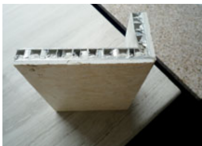
Fig. 4.5 – Aluminum honeycomb backing with thin marble.
