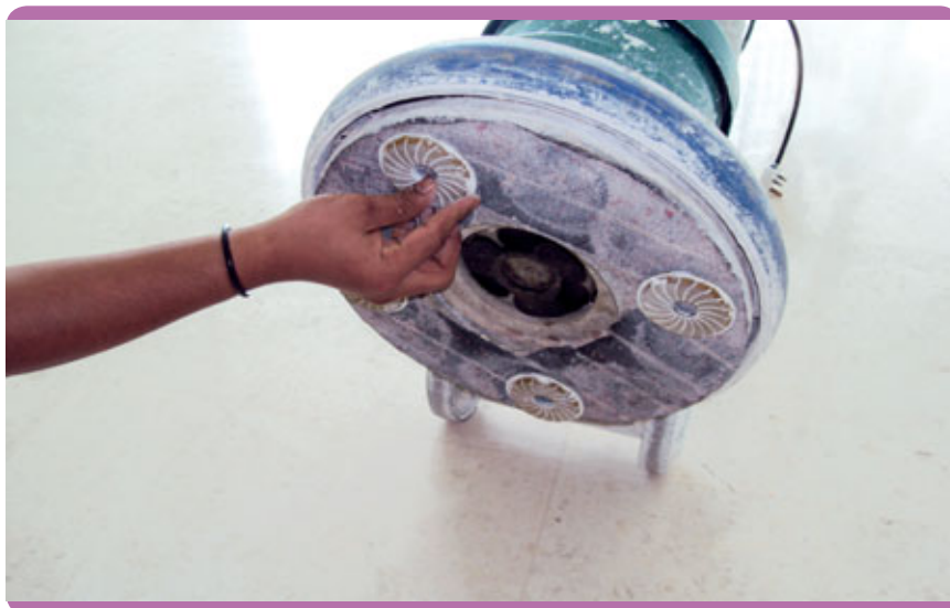
Fig. 1.7 – Polishing tools are similar to those for natural marble.
