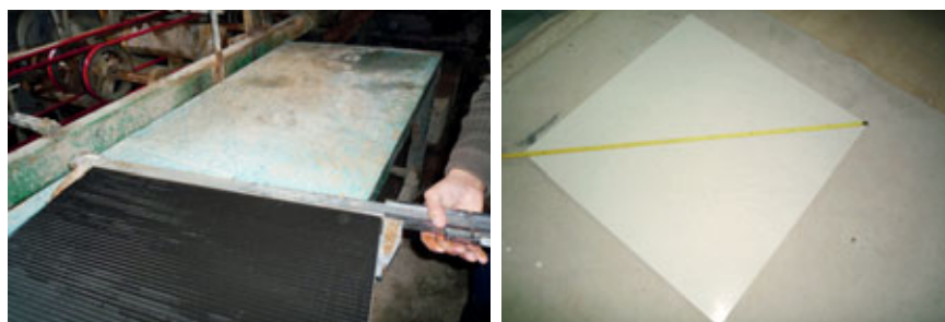
Fig. 3.2 – Size variation can be substantially minimized in rectified tile.
