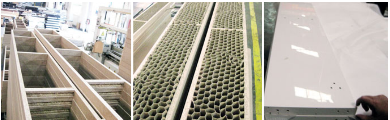
Fig. 10.6 – Tall and thin panels are possible using honeycomb infill.
