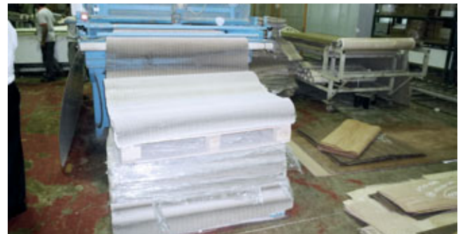
Fig. 10.5 – Honeycomb papers stretched mechanically and dried to achieve the desired strength.
