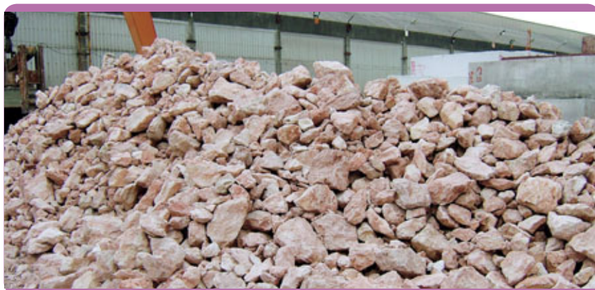
Fig. 1.1 – Raw material for agglomerated marble: Selected marble boulders.
