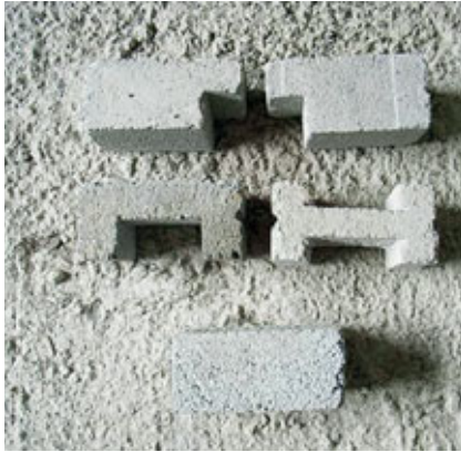
Fig. 13.2 – Different profiles of recessed blocks to embed pipes.
