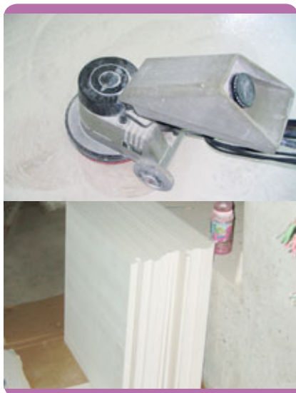
Fig. 1.6 – Homogeneous body can be repeatedly polished and renewed.
