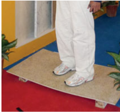
Fig. 4.3 – The backing technology yields better flexural strength.
