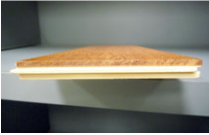
Fig. 8.1 – A typical section of engineered wood flooring strip.
