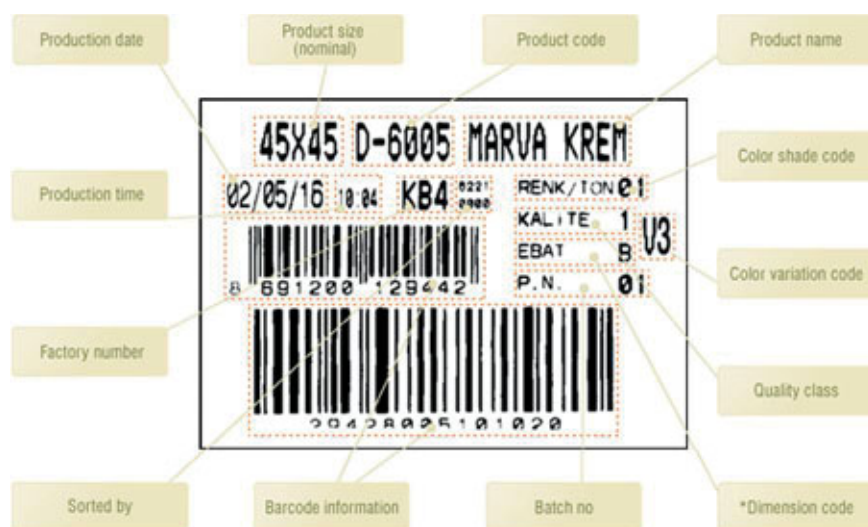
Fig. 3.13 – Typical information on tiles packing.
