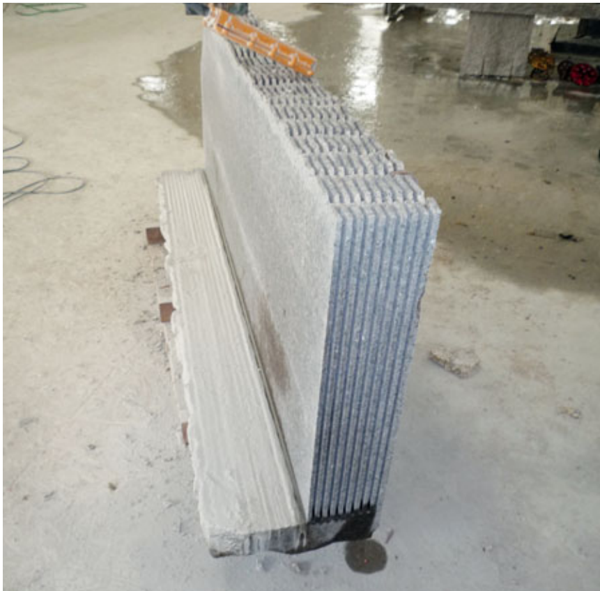
Fig. 4.4 – Thin cuts from same block increases utilization ratio.
