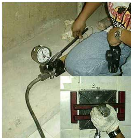
Tiling pull-off test
