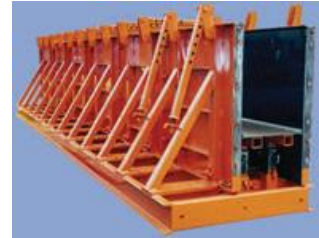
Fig 2.6 Example of adjustable mould for the precast beam and column production
