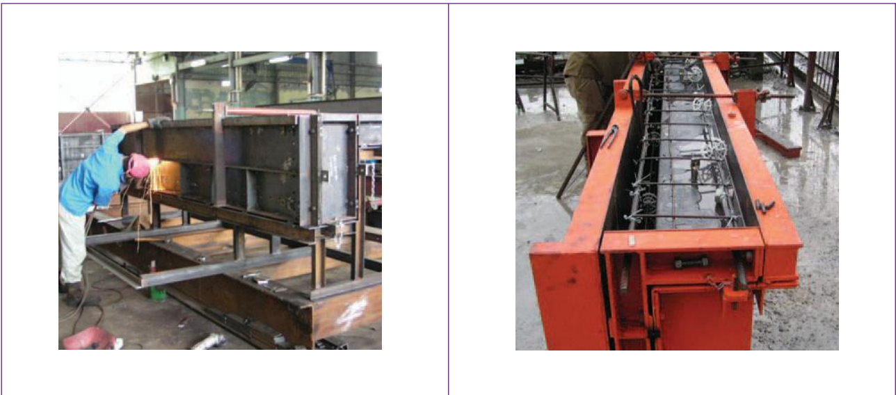
Figure 2.7 Adequate bracing is required for better dimensional controls
