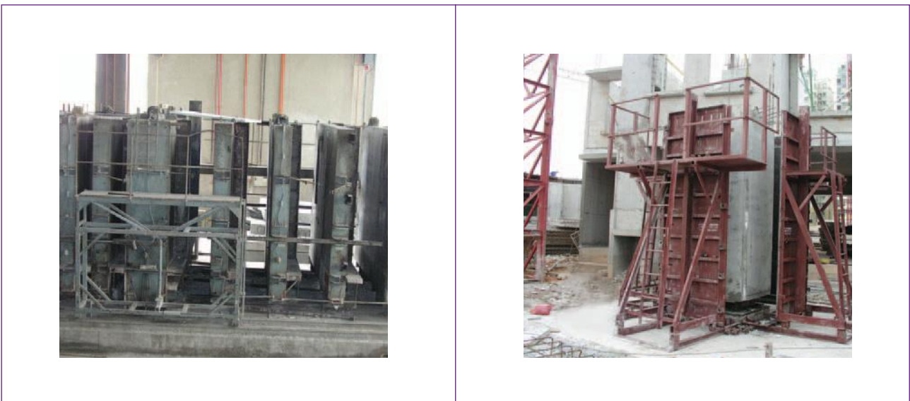
Figure 2.8 Examples of battery moulds and mechanised vertical moulds used for wall elements
