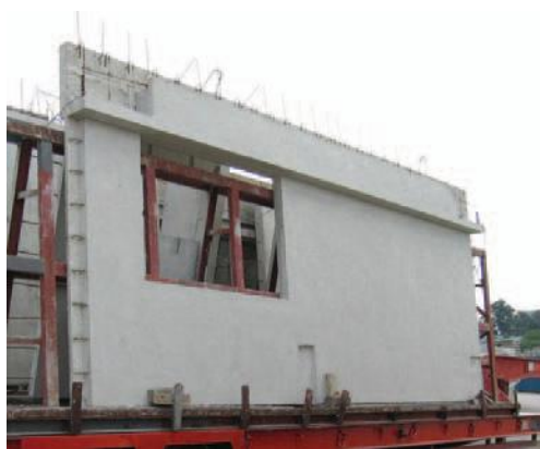
Figure 2.1 Integrated beam and wall panels
