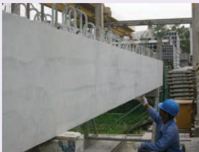
Finishing works before delivery to site
