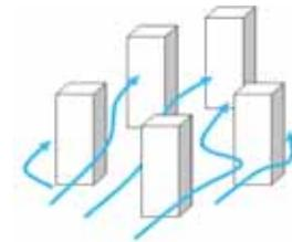
[Figure 14] Staggered arrangement of blocks with sufficient spacing between blocks.
