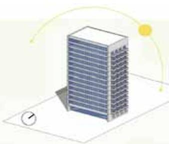
[Figure 16] Minimise solar heat gain by adding balconies as shading devices.
