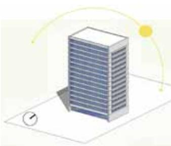
[Figure 15] Minimise solar heat gain by shading all the East or West façade openings.
