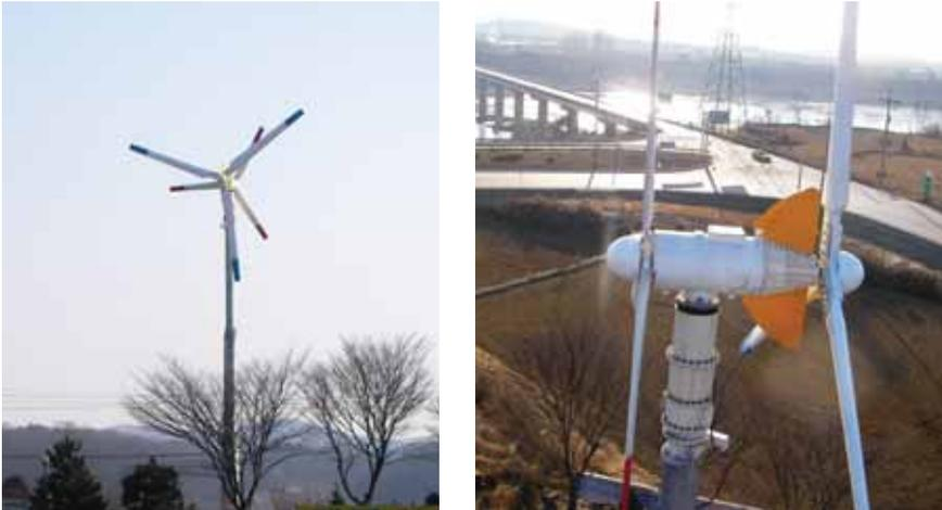
[Figure 2] Examples of Horizontal-axis wind turbines (HAWTs). 6 bladed wind turbine generator installed beside conventional 3 blade wind generator – near Bi-young Bridge at Kyunggi-Do South Korea.
