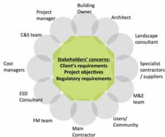
[Figure 1] Stakeholders typically found in a construction project.
