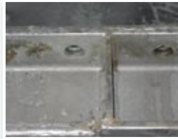
Stage 1: Blow-out from overlapping area on this fabrication has caused a galvanised coating defect
