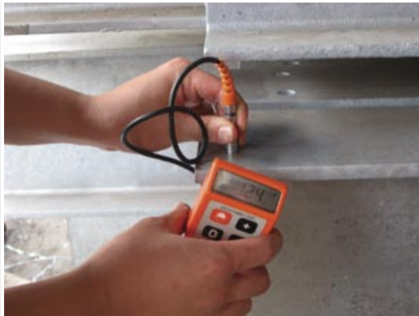
Coating thickness measurement (eddy current)
