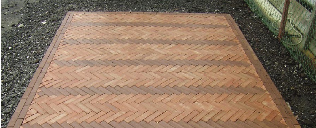
Figure 28. Concrete pavers made with ceramic aggregates
