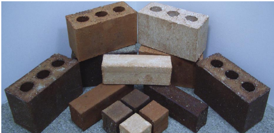
Figure 29. Concrete blocks and bricks manufactured with ceramic aggregates
