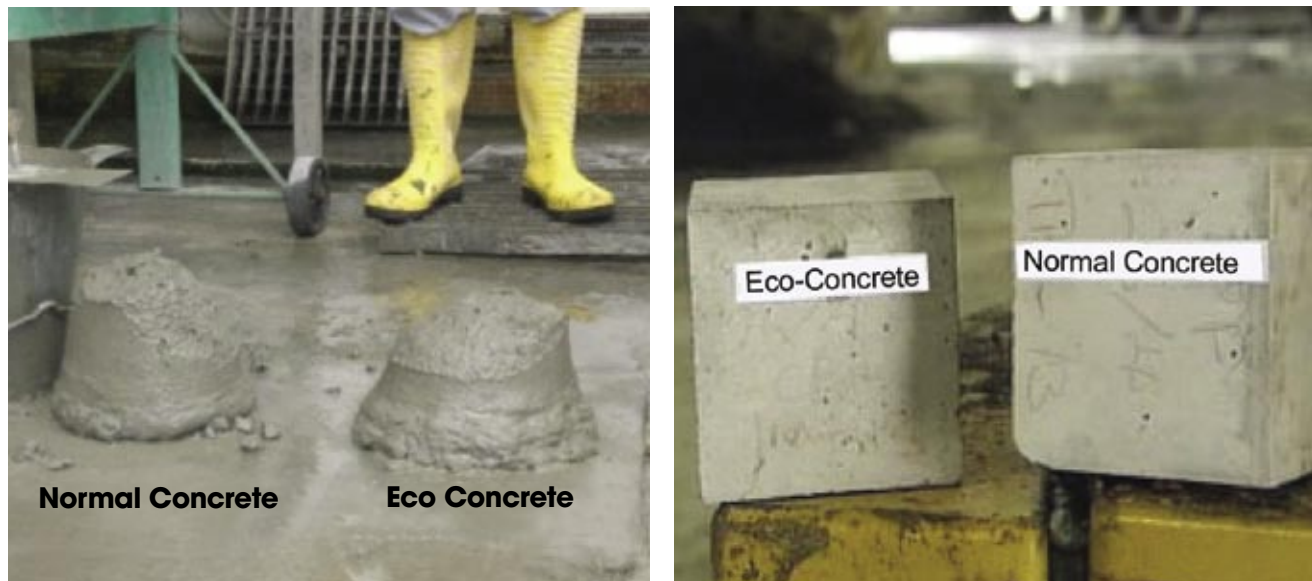
Figure 19. Conventional concrete compared to Eco-concrete
