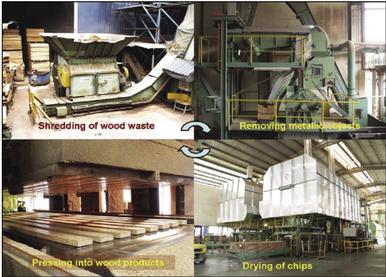
Figure 9. Process flow for converting wood waste into useable products
