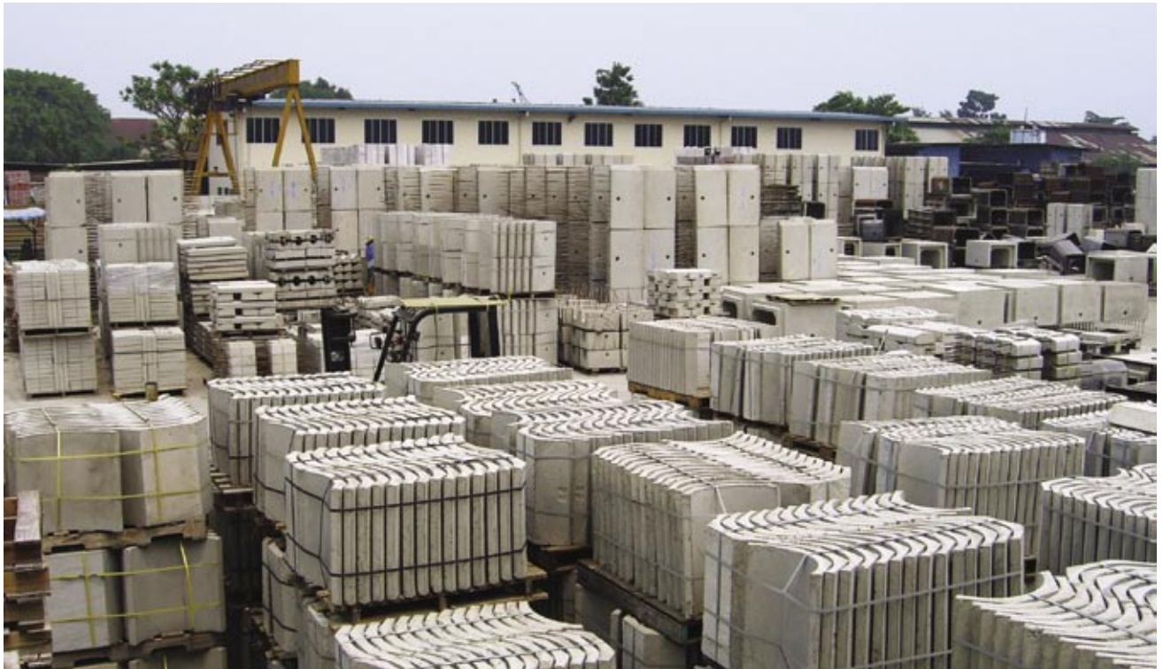
Figure 26. Precast concrete components with RCA
