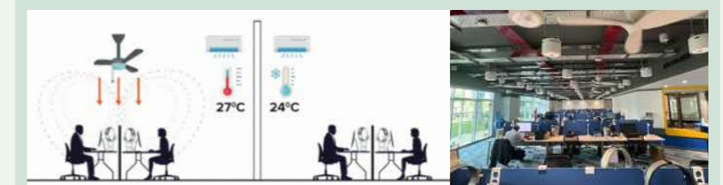
Hybrid cooling system tested at BCA's ZEB Plus office. The hybrid cooling system operates by raising the setpoint temperature of the office air-conditioning system from 24 to 26.5°C, and is supplemented by ceiling fans. In doing so, the ZEB Plus office can achieve 32% energy savings on the air-conditioning system while maintaining thermal comfort for its occupants.
