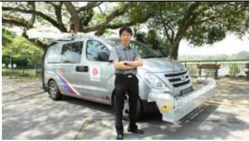
Samwoh adopted a productive crack measurement system which uses laser and image recognition technology to collect road condition data for road maintenance.
