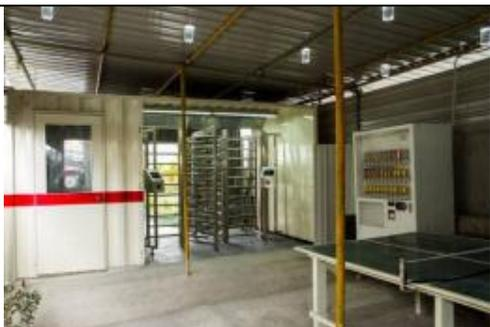
Straits Construction has adopted the Site Access System (SAS) which utilised biometric identification, a contactless facial scanner to regulate faster entry and exit at the site.
