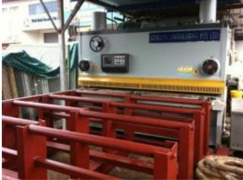
The automatic hydraulic shearing machine it purchased with funding support from the BCA Construction Productivity and Capability Fund produces better quality work and also reduced manpower required.
