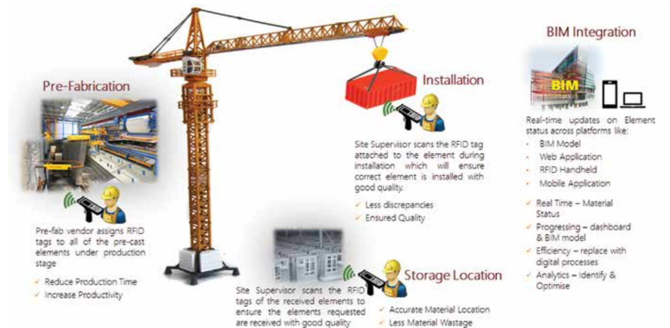
An illustration of how the materials tracking solution works
