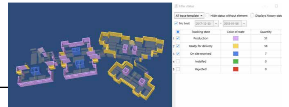
A screenshot showing how each element is reflected on the system in real time, keeping users updated on the status of each precast component
