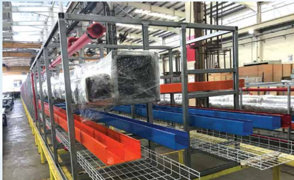
An example of prefab MEP horizontal ceiling modules
