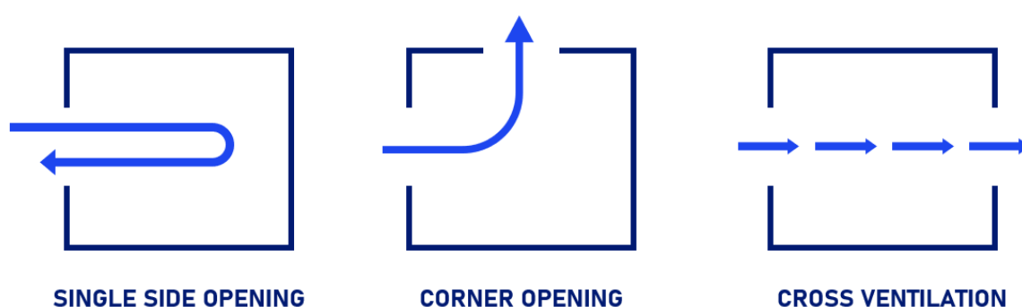
Figure 3 Types of Window Configuration
