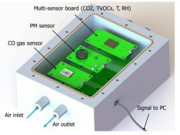
The prototype with novel low-cost sensors for IEQ monitoring and characterisation
