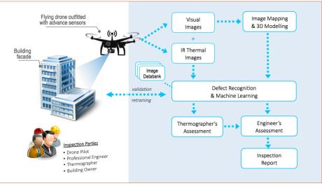
Figure 2: Drone Inspection Workflow
