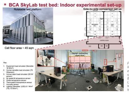
Figure 1: Indoor experimental set-up for Blinds and Lighting technology tests
