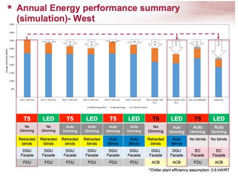
Figure 3: Annual Energy performance summary (simulation) for all combination technologies - West orientation
