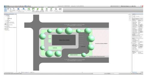
This project aims to develop Building Information Modelling (BIM) auto-checker plugins based on NParks regulatory requirements as well as uncover the necessary object parameters to be included in order for these checkers to work. For example, vegetation objects need to have a Leaf Area Index (LAI) parameter in order the Green Plot Ratio (GnPR) to be calculated.
