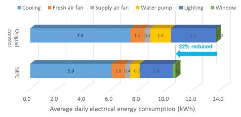
Figure 2. Energy performance of developed MPC system as compared to conventional BMS
