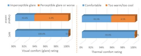
Figure 3. Thermal and visual comfort of developed MPC system as compared to conventional BMS
