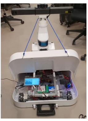
This project aims to develop an autonomous self-navigating robot, which can be used for inspection of buildings. Equipped with state-of-the-art technologies including computer vision and sensor fusion, coupled with high resolution camera for inspection, the robot can also read information from Building Information Modelling (BIM).
