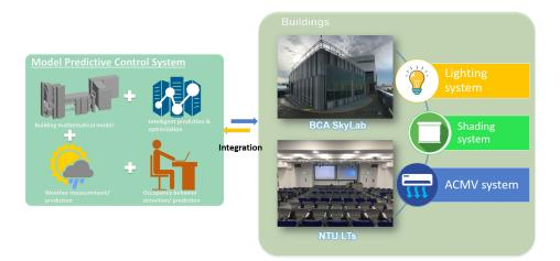
Figure 1. Schematic of MPC system and integration with buildings
