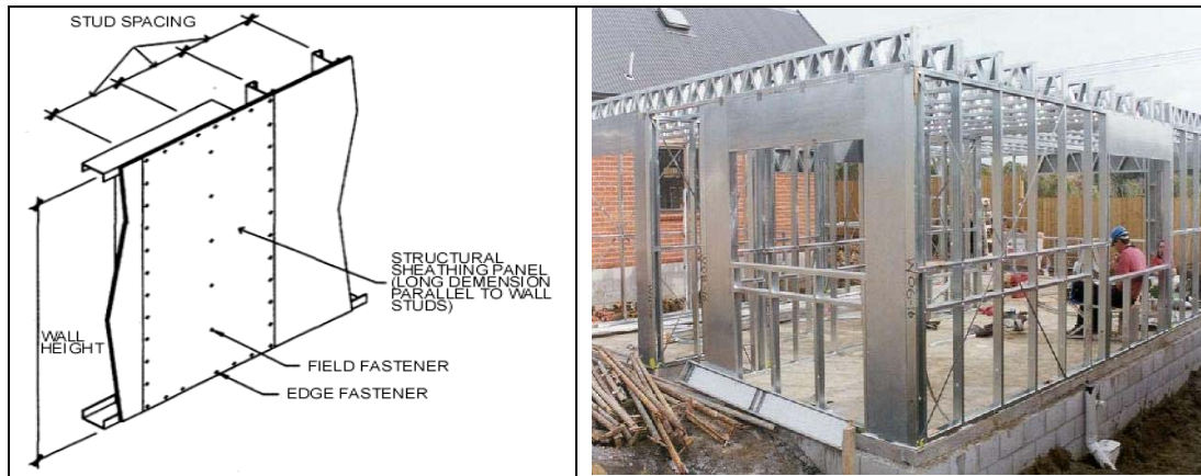
Figure 10.5 Structural Sheathing Fastening Pattern
