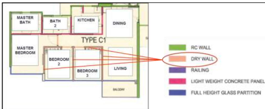
Figure 1 – Example of a layout showing the mandatory use of drywall for all internal dry areas.
