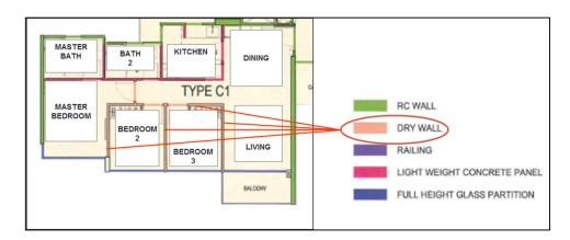
Figure 1 – Example of a layout showing the mandatory use of drywall for all internal dry areas.
