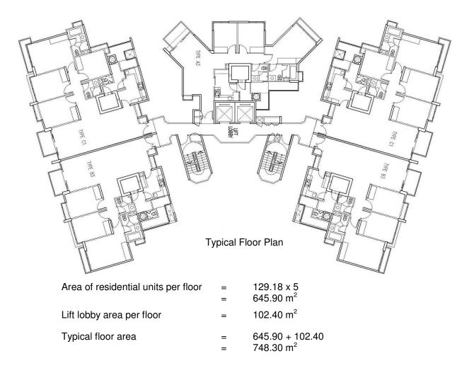
Design based on flat plate system with cast in-situ columns with wall combination of precast walls and dry wall.
