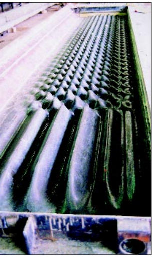
Computer-patterned concrete mould used for the façade panels on the National Museum, Canberra Images courtesy of : Photocall Australia
