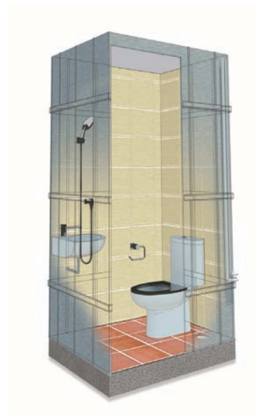
Stage 4- Install sanitary wares such as basin and water closet. Once PBU is completed, it is protected and ready for delivery to site
