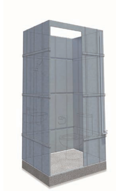
Stage 2 - The wall is made of galvanised steel sheets and assembled together with steel frames. Mechanical and Electrical (M&E) services are installed at this stage
