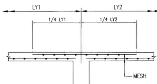
TYPICAL DETAIL IN THE SECONDARY DIRECTION
