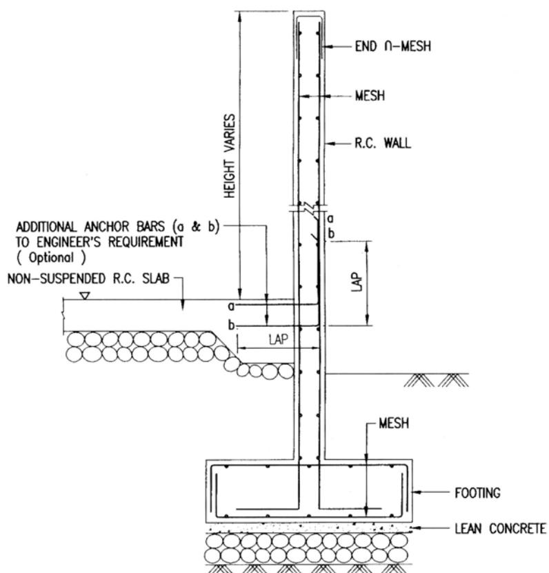
The meshes are simply laid in the trench on suitable spacers. The mesh width allows for a generous side cover to the cross wires.
