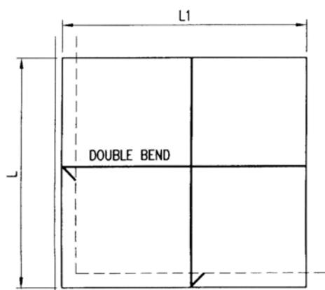
Plan of Top Reinforcement at Slab
