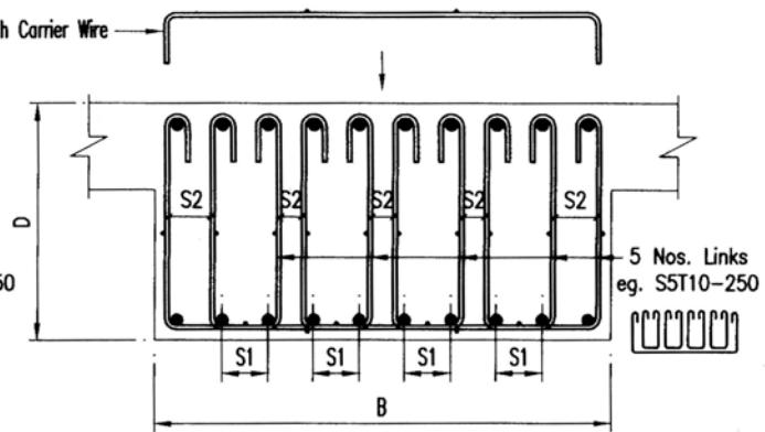
NOTE: (1) Internal links shall not overlap as shown in the diagram.
