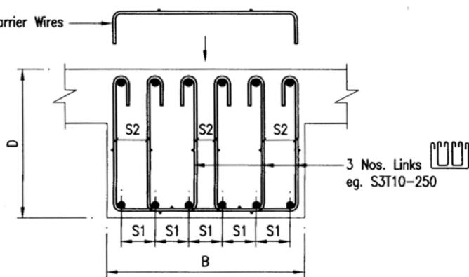
Example '5' (For  $750\text{mm} < B < 950\text{mm}$ )
