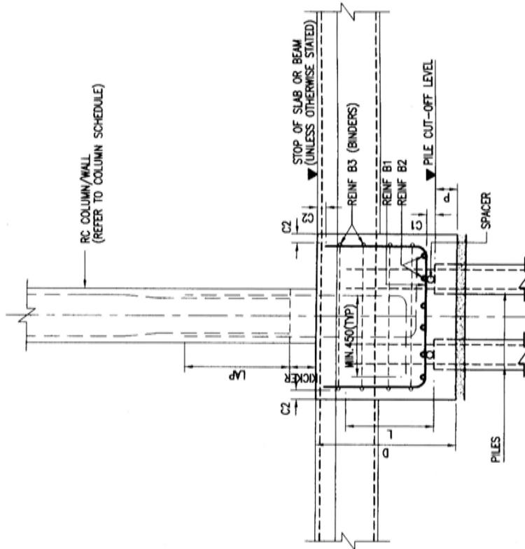
Example '2' : Typical Pilecap Sectional Detail with Slab or Beam Case Together
