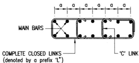
2. ALL ALTERNATE MAIN BARS SHALL BE TIED BY 'C' LINKS IF THE SPACING EXCEEDS 150mm ( FOR  $b > 150\text{mm}$  )
