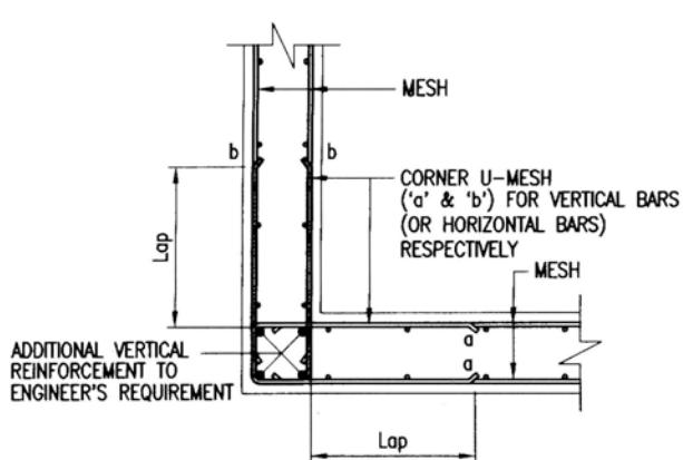
Typical Wall Corner Reinforcement Detail
