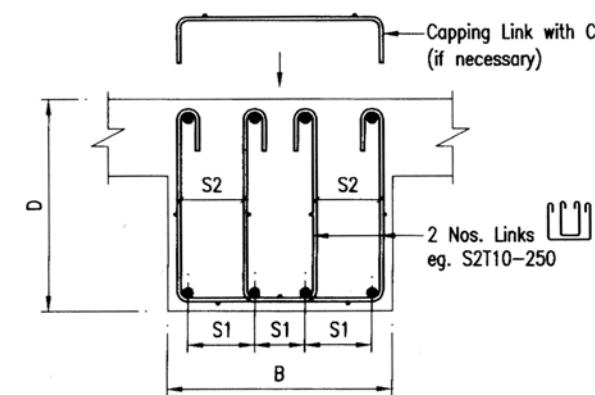
Example '4' (For  $600\text{mm} < B < 750\text{mm}$ )
