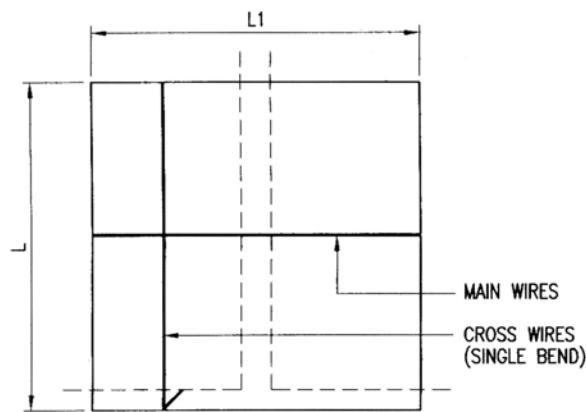
Plan of Top Reinforcement at Slab
