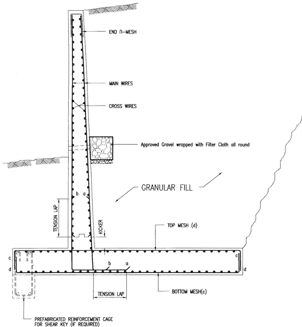
**EXAMPLE (2) : TYPICAL SECTION OF RETAINING WALL**
