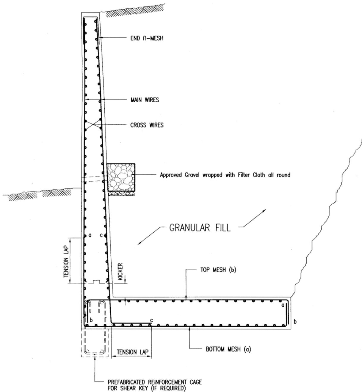
**EXAMPLE (1) : TYPICAL SECTION OF RETAINING WALL**
