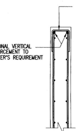
Typical Wall End Reinforcement Detail
