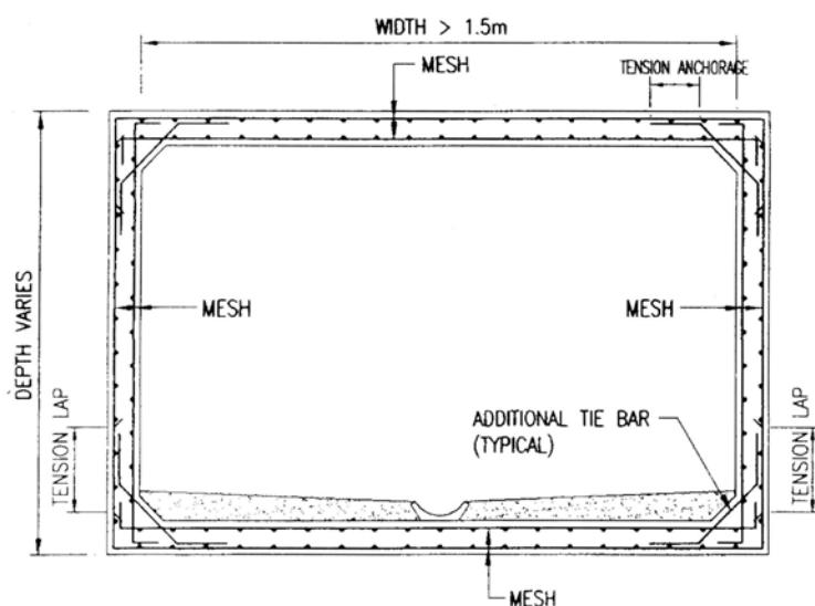
TYPICAL SECTION FOR LARGE SIZE CLOSED DRAIN
