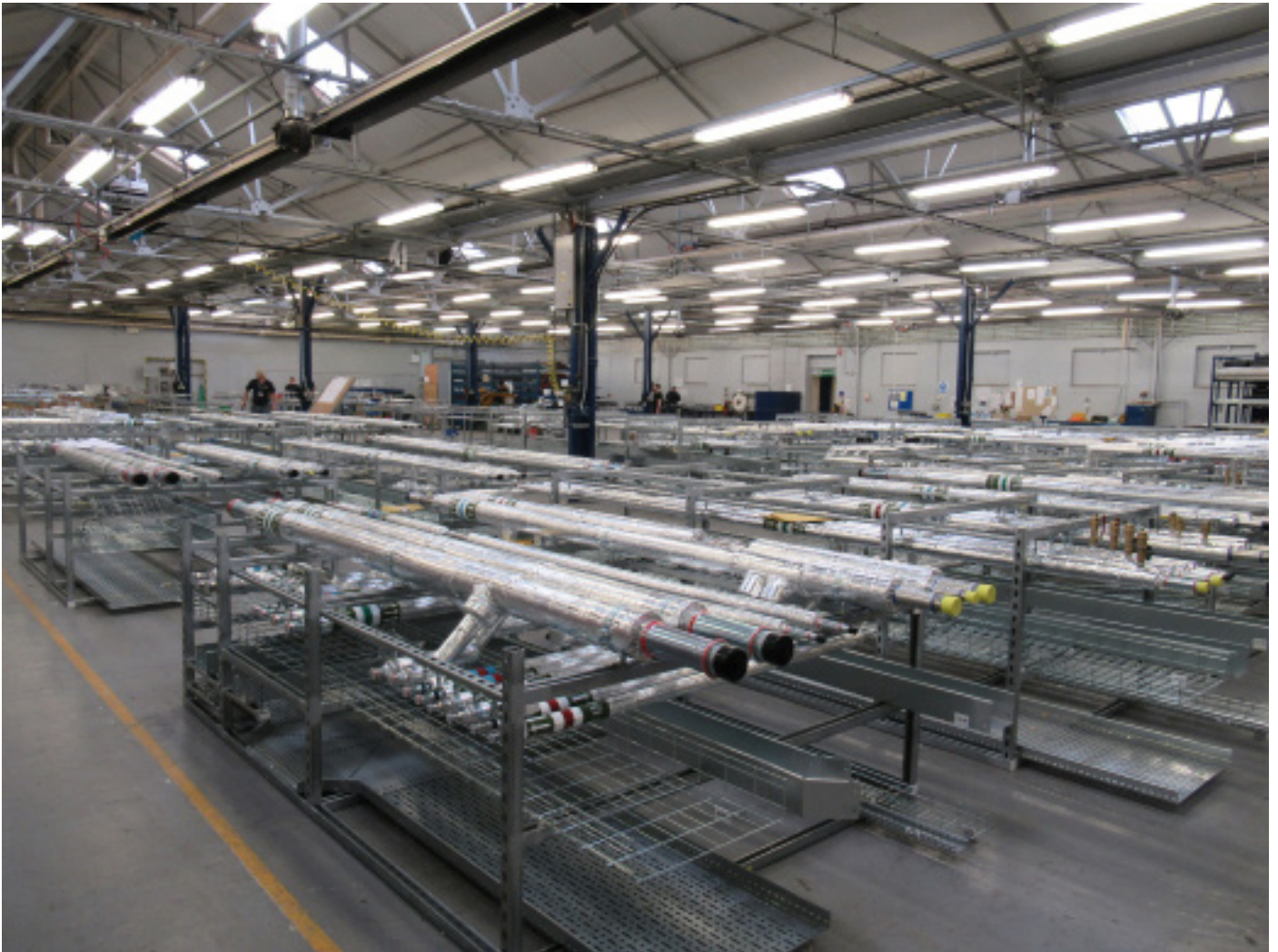
Figure 12: Alignment of modules in a factory. Prefabricated MEP modules are fitted out in the factory, prior to delivery and installation on site ( Photograph courtesy of DSG Modular )
