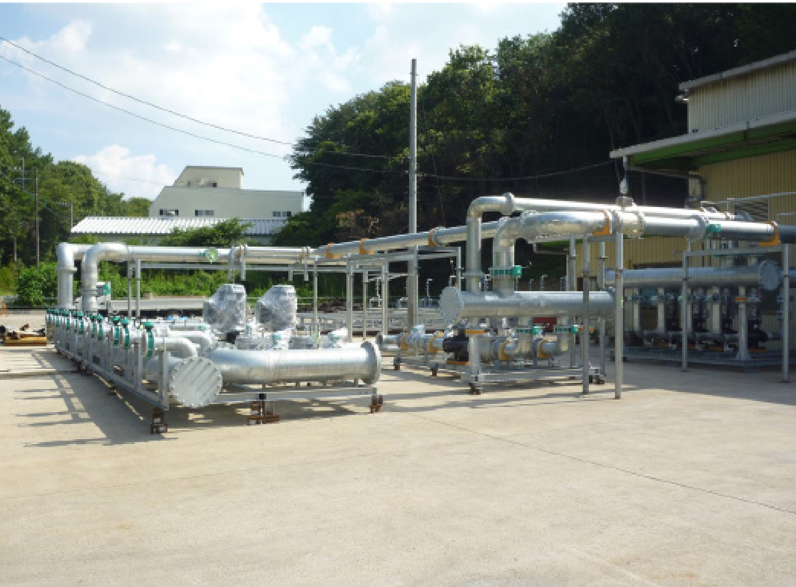
Figure 11: Prefabricated plant modules fitted and lined up in factory (Photograph courtesy of Seikei factory, Japan)
