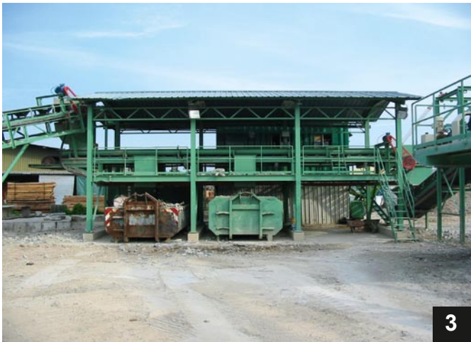
Removal of foreign materials such as bricks, plastics and asphalt
