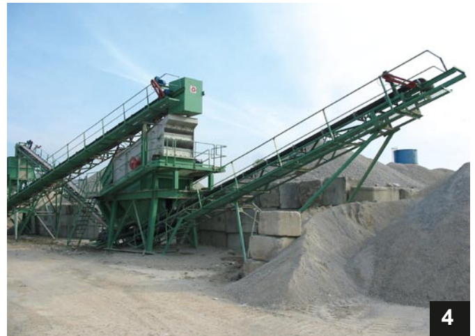
Further crushing and screening of RCA into various sizes
