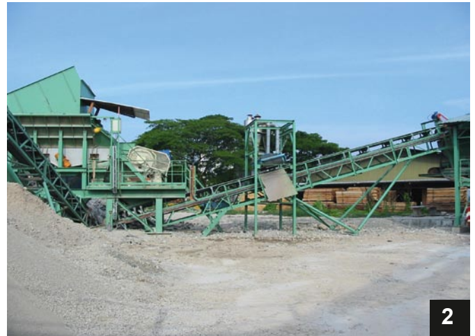
Preliminary crushing and removal of ferrous metals
