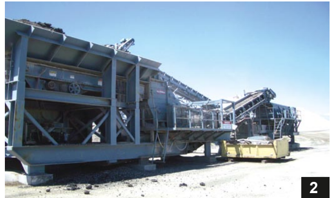
Crushing and screening of asphalt pavement waste
