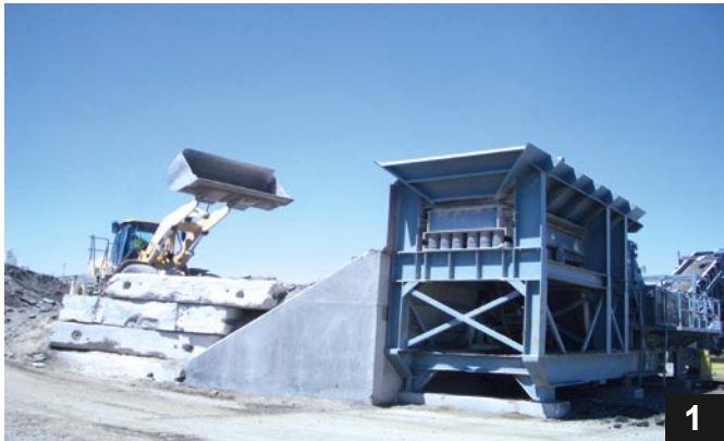
Loading of asphalt pavement waste for crushing
