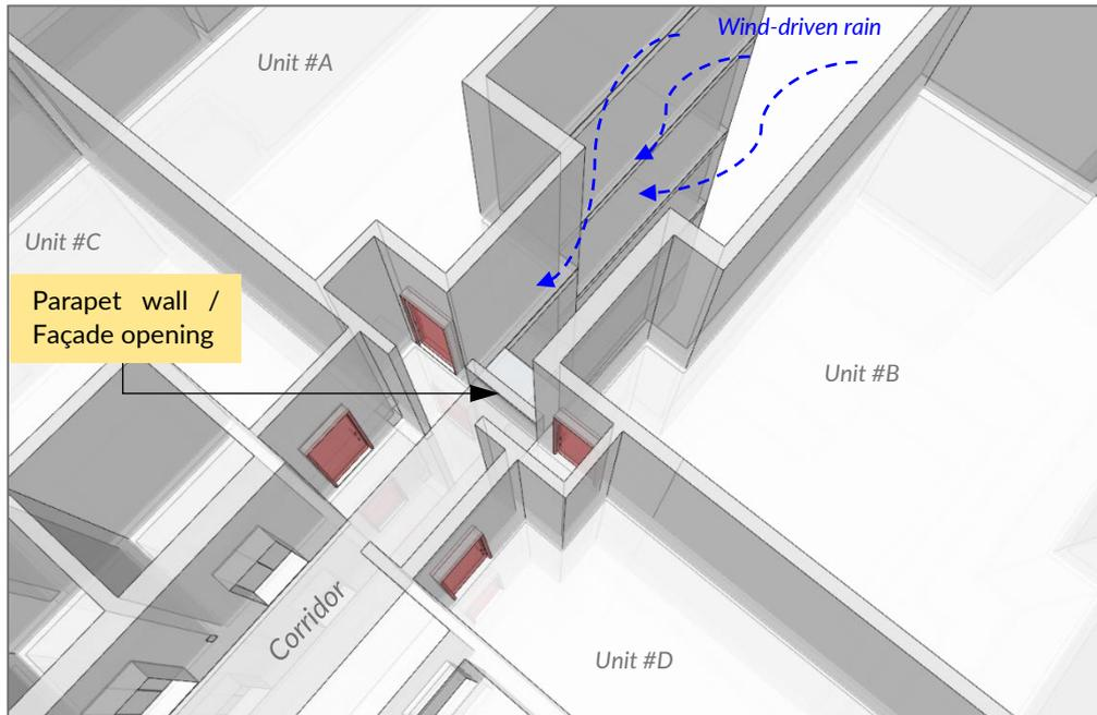
Figure 11: Diagram showing unit entrances (#A & #B) oriented away from façade opening
