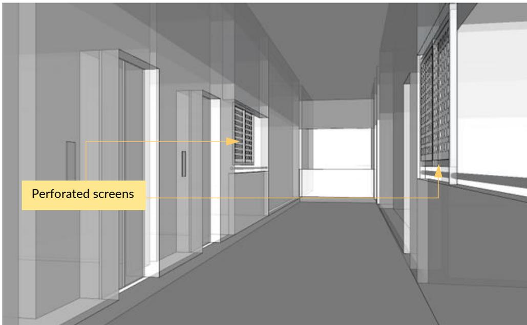
Figure 9: Provision of perforated panels along long cross-ventilated corridors
