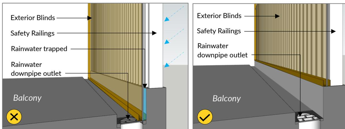
Figure 15: Cross-sectional view of exterior blind installations
