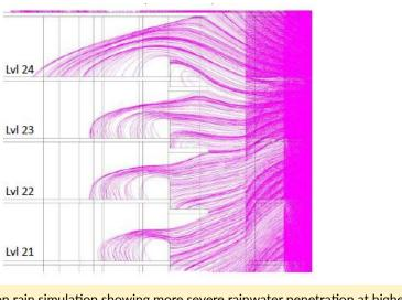
Figure 6: Wind-driven rain simulation showing more severe rainwater penetration at higher levels
