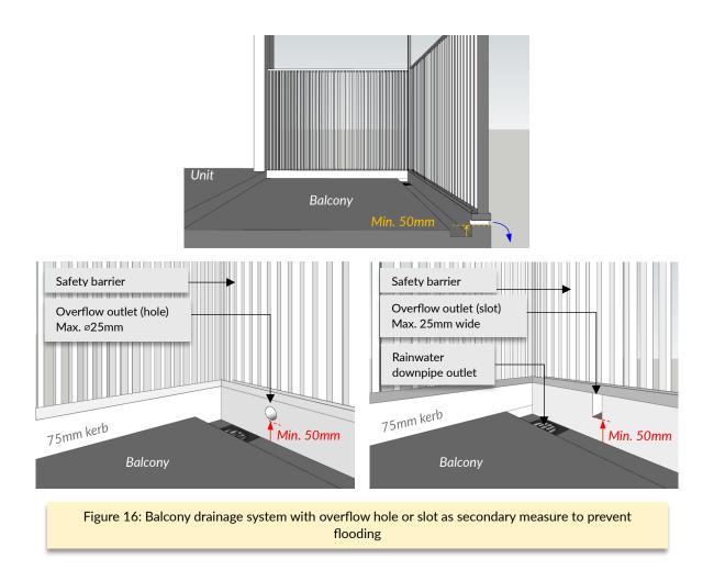
During heavy rainfall, the existing drainage system may prove inadequate to manage the volume of water, resulting in significant ingress and ponding issues, particularly in balconies and corridors. This problem primarily arises from insufficient capacity in rainwater downpipes (RWDP) and a lack of properly sized or adequate number of rainwater outlets (RWO). Poor drainage system design may also contribute to the issue.
