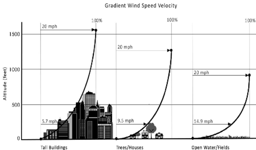
Figure 5: Variation of mean wind velocity profile with surface roughness
