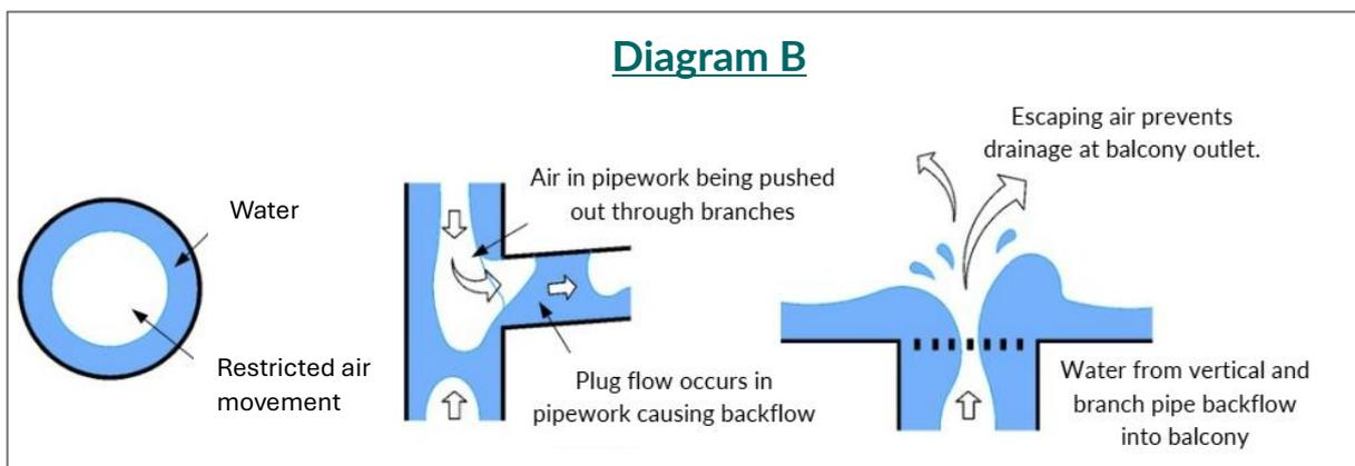
Figure 24: Under-Design of Balcony Drainage System causing Backflow
