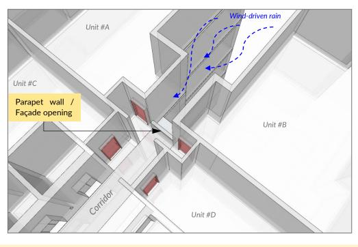
Figure 11: Diagram showing unit entrances (#A &#B) oriented away from façade opening
