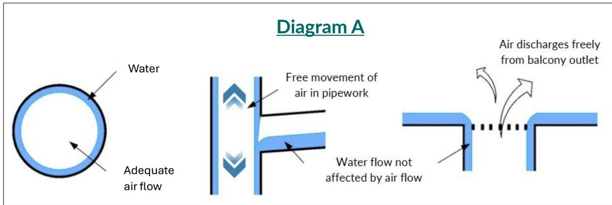
Figure 23: Correct Design of Balcony Drainage System
