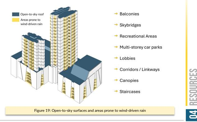
The number of scupper outlets needed for effective drainage in common areas will be determined by the surface area in contact with rainwater, the rainfall intensity, and the size of scupper drains provided. Designers must evaluate the flow rate (rate of run-off) in areas potentially exposed to wind-driven rain. This assessment is crucial for strategically placing outlets and scuppers, and for providing sufficiently sized pipes to ensure effective rainwater drainage.
