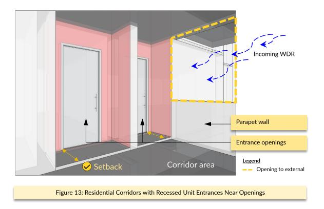
**Door gates:** Gates if any, should be designed with appropriate porosity in response to the expected rain ingress at the unit entrances.
