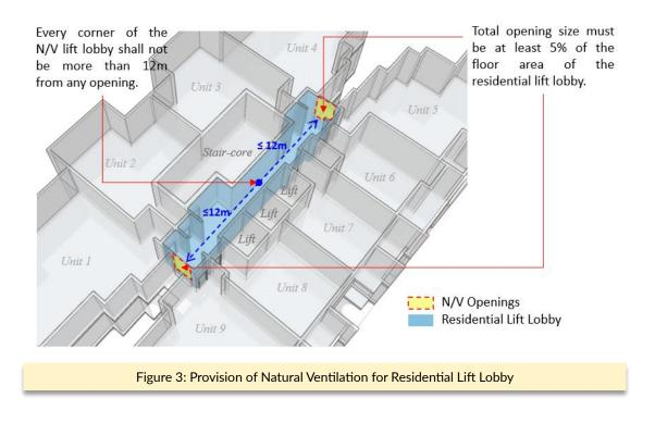
In terms of fire safety, ventilation openings are essential to facilitate smoke dispersal, reduce the likelihood of the corridor being smoke logged, as well as minimise smoke entry into the exit staircase when used by evacuees and emergency responders during fire emergencies.
