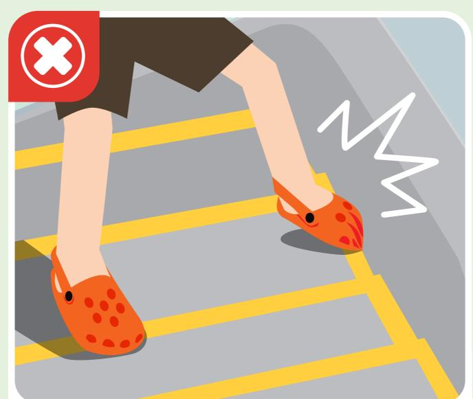
Do not stand near the sides of the escalator. Soft footwear may get stuck in between the gaps in the escalator. 请勿站靠近梯级边缘。穿着软鞋类的乘客请多注意梯级边缘、梳齿板等的细缝,以免鞋子被夹住。
