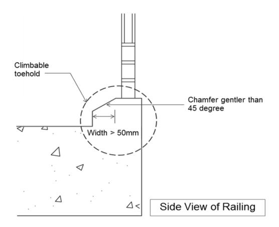
Figure H.3.4A.1(d) – Toehold Dimensions at Kerb/ Protrusion
