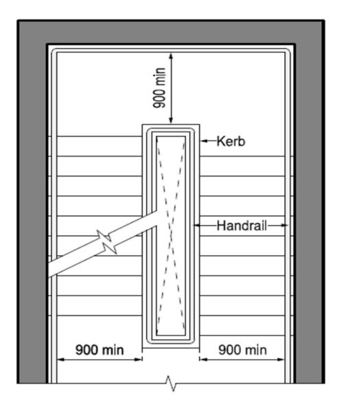
Figure E.3.5.3(a) Measurement of landing width
