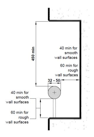
Figure E.3.6.4(a) - Handrail in Recess
