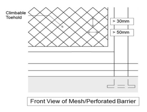
Figure H.3.4A.1(b) - Toehold Dimensions at Mesh/Perforated Barrier
