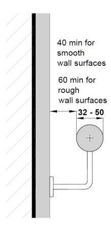
Figure E.3.6.3(a) – Handrails Clearance from Wall
