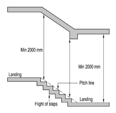
Figure C.3.2.1(a) - Measurement of Headroom
