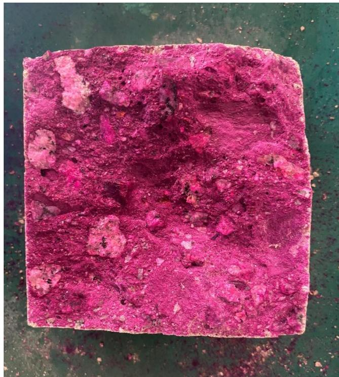
Figure 17. Carbonation depth of the 100%-GF mix after 20 months' exposure to natural condition
