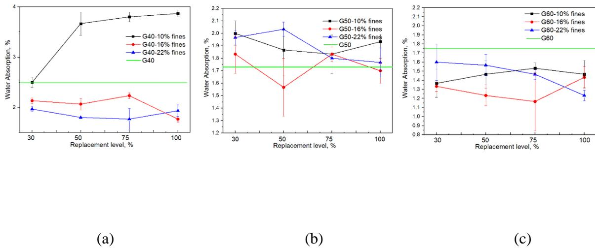
Figure 6. Water Absorption (a) G40; (b) G50; (c) G60
