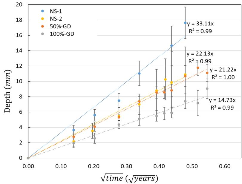
Figure 14. Carbonation depth in accelerated test condition
