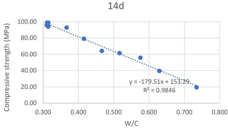
Figure 3. The relationship between compressive strength and W/C at 14 days
