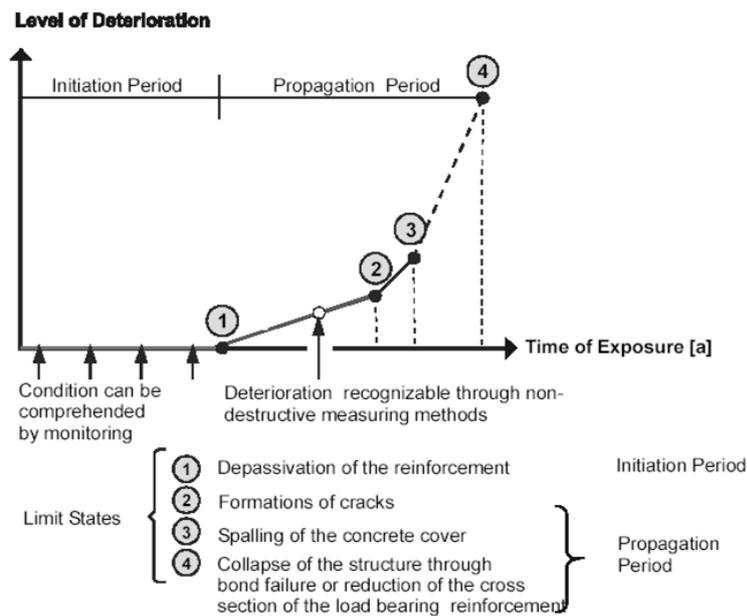
Figure 18. Typical deterioration levels for a steel reinforced concrete structure suffering from reinforcement steel corrosion<sup>10</sup>
