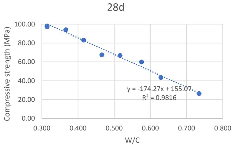
Figure 4. The relationship between compressive strength and W/C at 28 days
