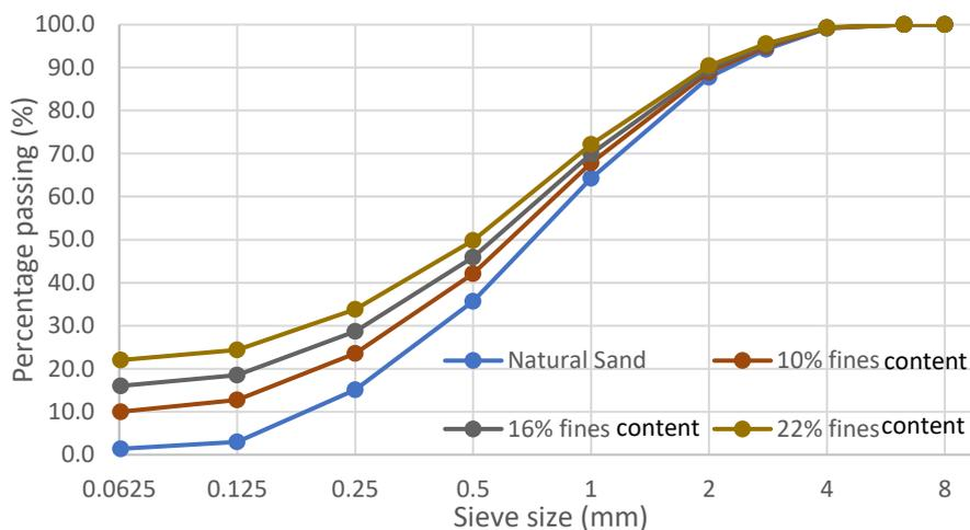
Figure 1. Gradation of Natural Sand and Produced Sample
