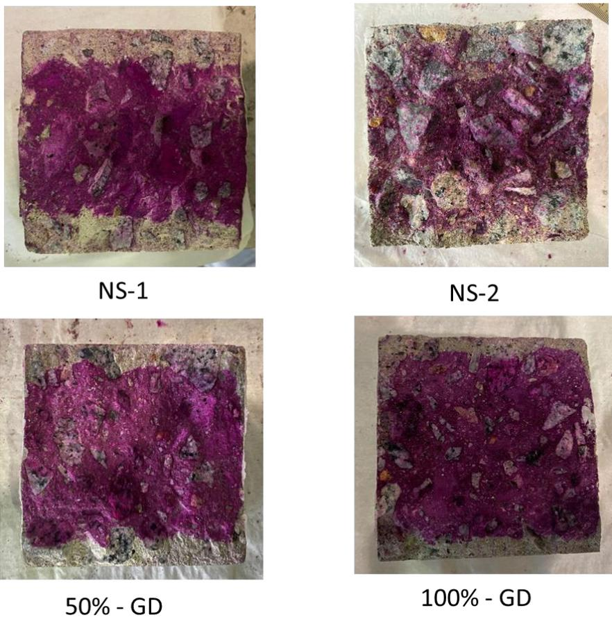
Figure 15. The carbonation pattern for the 84-day measurement of the accelerated test
