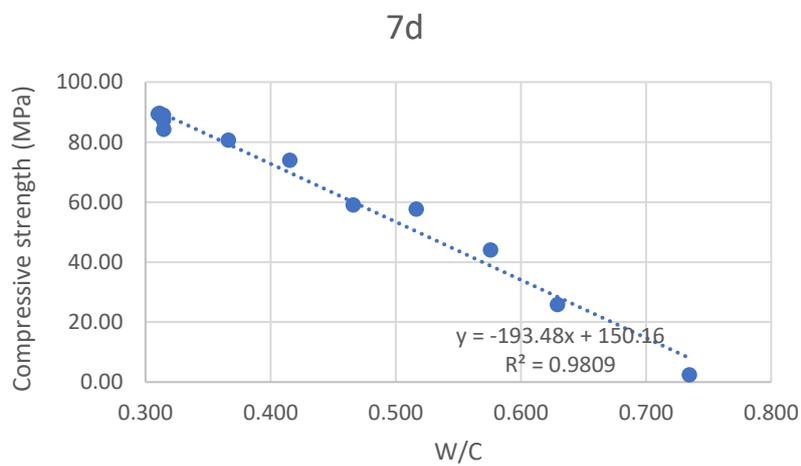
Figure 2. The relationship between compressive strength and W/C at 7 days
