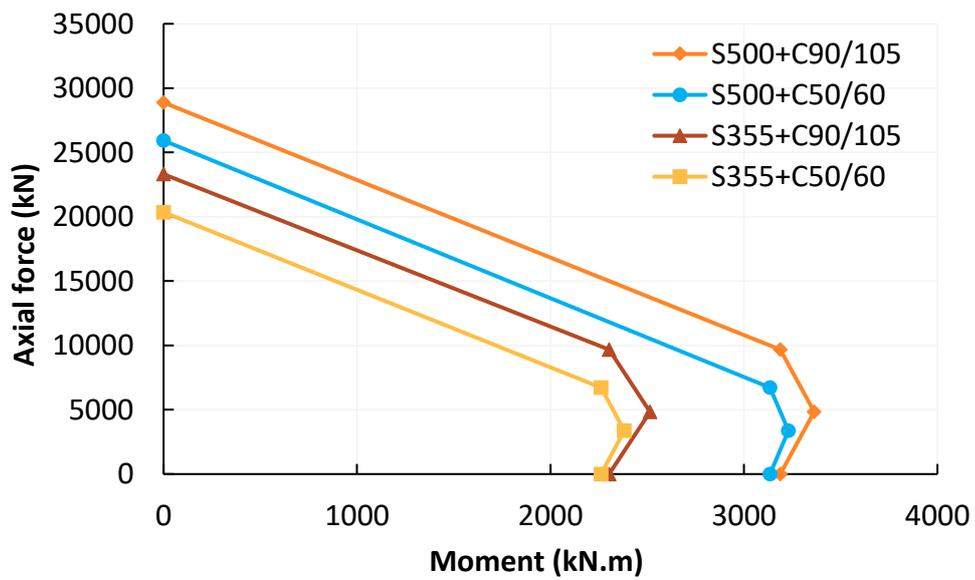
Figure 15: Design M-N interaction curves about z-z axis
