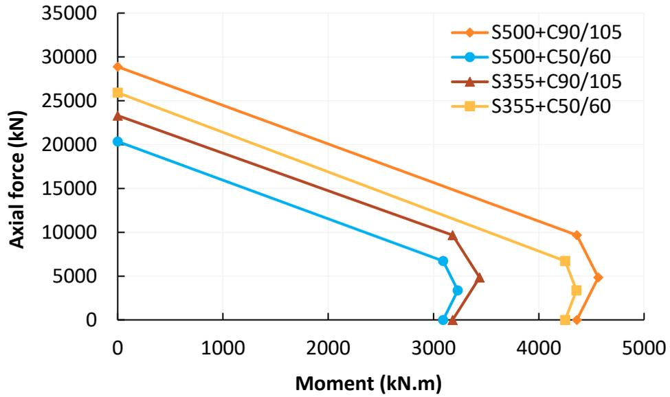
Figure 14: Design M-N interaction curves about y-y axis
