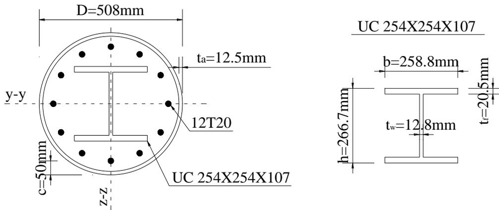
**Figure 3: Cross-sectional dimensions of CFST column in Example 2**
