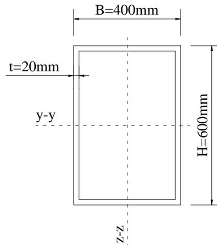
**Figure 9: Cross-sectional dimensions of CFST column in Example 3**
