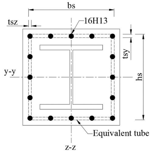
$$t_{sy} = 5(\pi/4)d^2 / (b_c - 2cs) = 5(\pi/4) \times 13^2 / (400 - 2 \times 30) = 2 \text{ mm}$$
