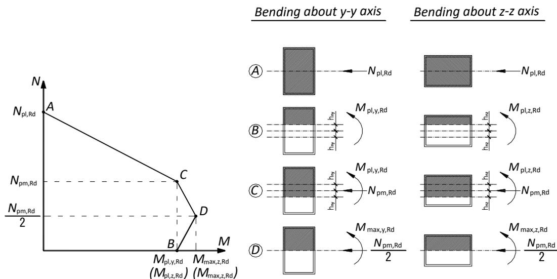
**Figure 10: Simplified interaction curve for rectangular CFST columns**
