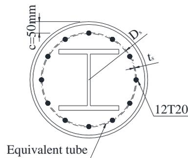
**Figure 4: Equivalent tube section for reinforcing steel**
