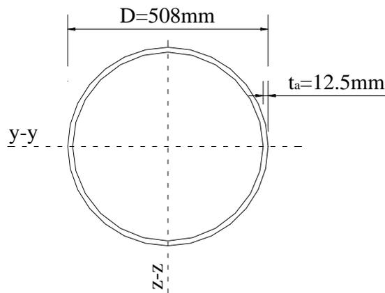
**Figure 1: Cross-sectional dimensions of CFST column in Example 1**
