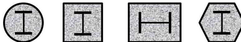
(c) Concrete filled steel tubes with an encased steel section
