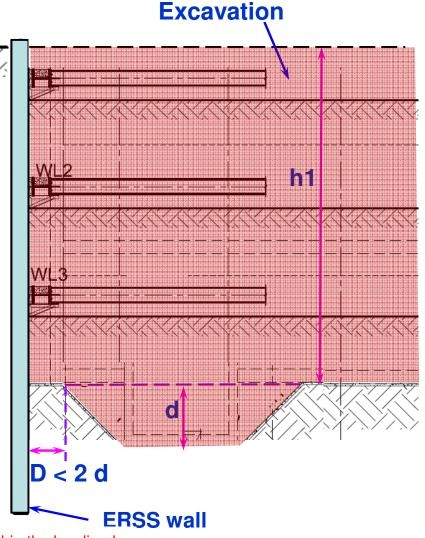
Note 1: localised excavation where the area of the structure within the localised excavation does not exceed 10 square meter and the width of the localised excavation parallel to the main ERSS wall/boundary not more than 5 m and depth not more than 2 m will be excluded from the computation of GBW.
