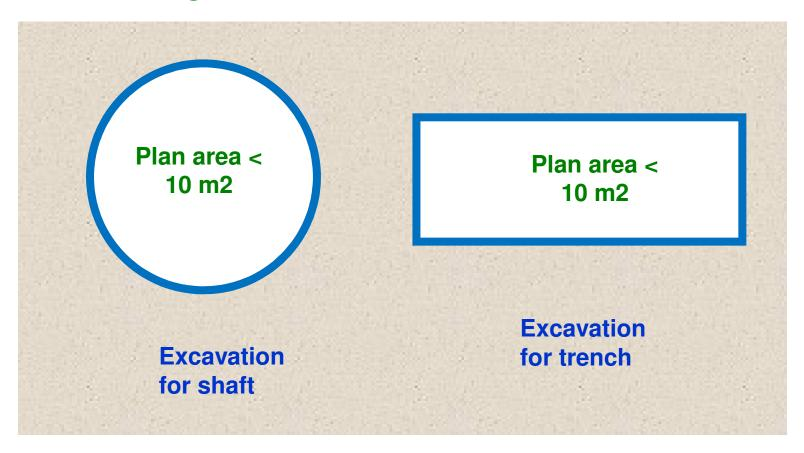
Any excavation for shaft and trenches with plan area of the excavation not exceeding 10 square metres (e.g. trench excavation for diaphragm wall, excavation for bored piles) is exempted from the requirements of geotechnical building works (GBW). For example, an excavation for a small shaft with plan area less than 10 sq m is exempted from the requirement of GBW but still subjected to ERSS submission requirements.
