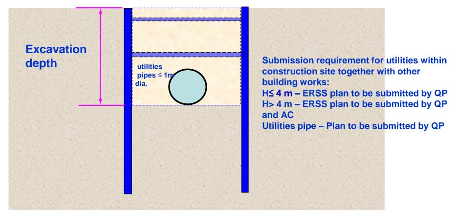
Any trenches for the purpose of laying sewers/utilities (including its associated shaft or manholes) not exceeding 1m in diameter in conjunction with any public sewerage/utilities system is classified as insignificant work which requires no plan submission. This exemption does not apply to cases where the trenches for the purpose of laying sewers/utilities (diameter less than 1m) are within a construction site where the size of trench exceeds 10 square metres or exceeds 2m in depth.
