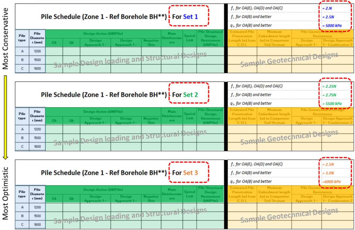
Fig A.2 – Sample of pile schedule showing 3 sets of pile design and parameters for project adopting performance-based pile design, submitted by QP(D) for ST approval
