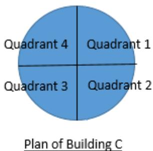
Building C, with a total height of H, has a circular plan with diameter D. The minimum coverage of the “Close-range” inspection shall be 10% of  $(\pi \cdot 0.25 \cdot D \cdot H)$  for each quadrant, and to cover all 4 quadrants of the building.
