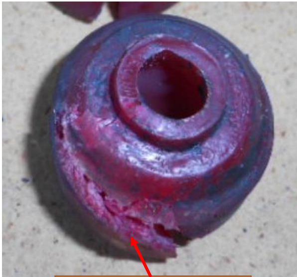
Damaged / Brittle PU Buffer
