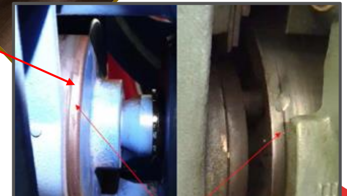
5. Contaminated Brake Drum (Oil Stain)
