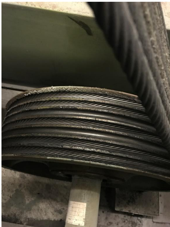
Excessive wear on deflector sheave
