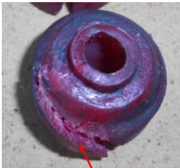
PU Buffer in Deteriorating Condition
