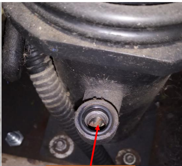
Insufficient Hydraulic Oil
