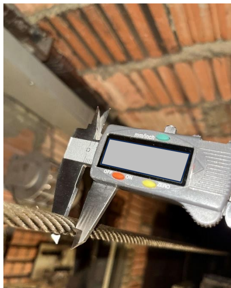
Governor rope diameter measurement
