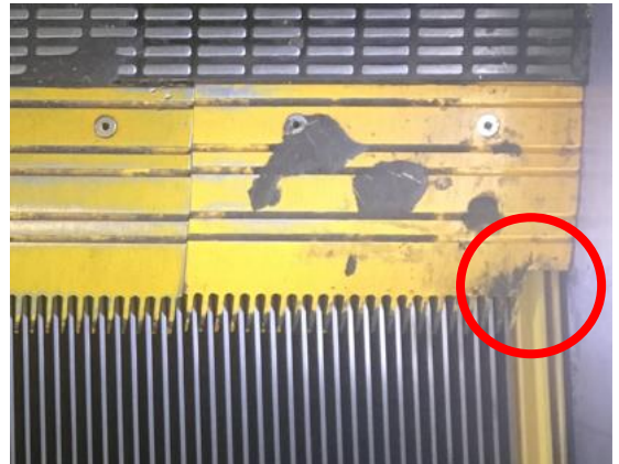
Consecutive broken teeth on escalator comb
