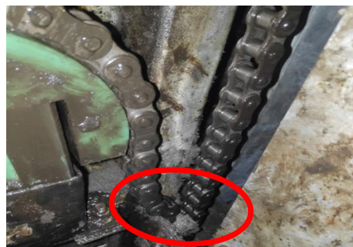
Broken handrail drive chain
