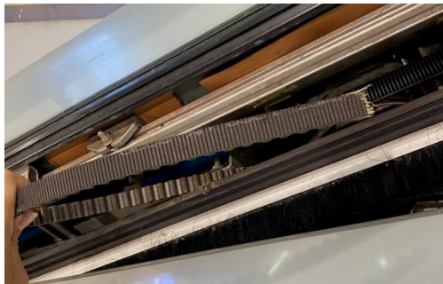
Broken handrail drive belt
