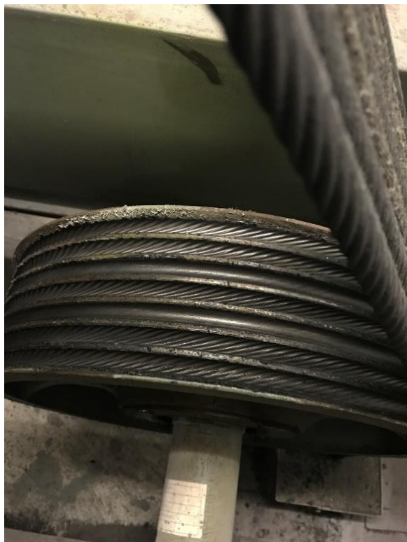
Excessive wear on deflector sheave
