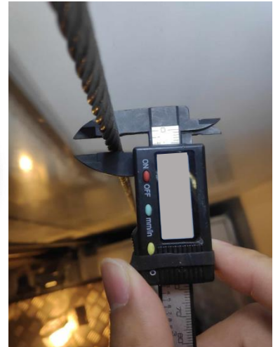
Governor rope diameter measurement
