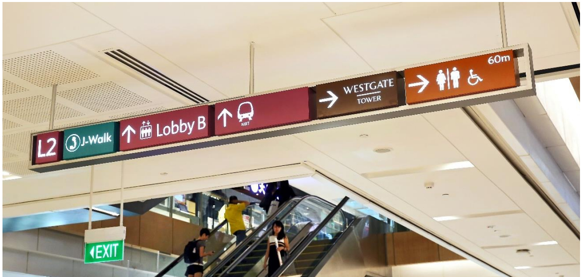
Photo (above): Example of signage with pictograms and distance to accessible features such as toilets.
