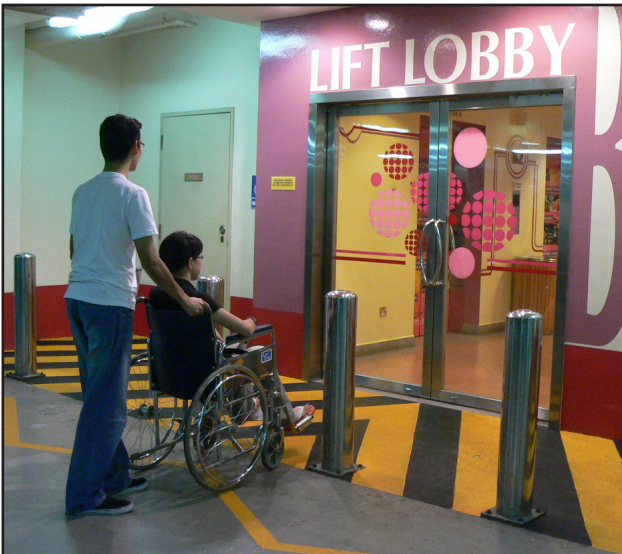
Adequate spacing between bollards to allow easy access by wheelchair users
