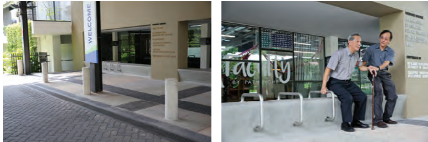
Photos (above): Examples of an accessible alighting and boarding bay, with suitable buffer zones and seats with armrests
