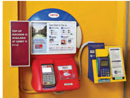
Photo (above): Controls and operating mechanisms with contrasting colours, as well as clear and logical instructions
