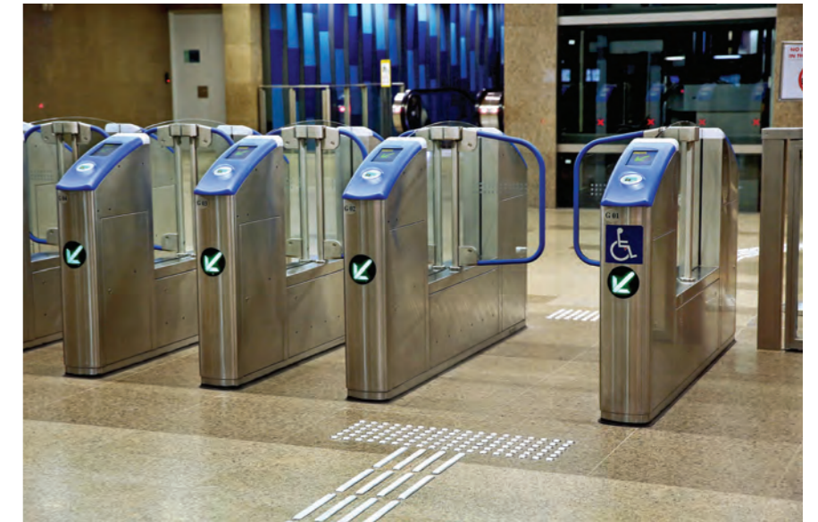
Photos (right and below): An accessible automatic fare collection gate; example of a lift that is readily identifiable
