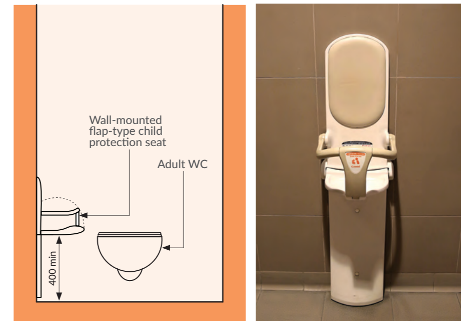
Figure 38. Front elevation of child protection seat in WC compartment
